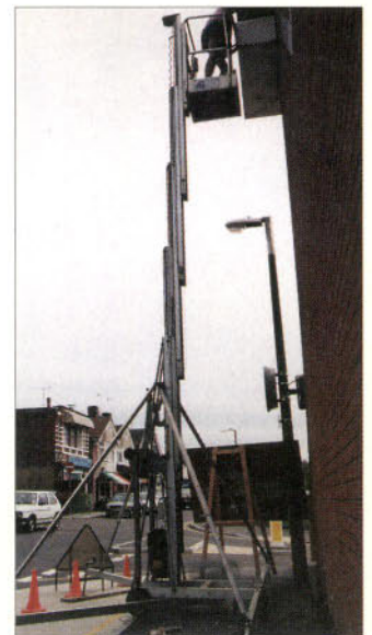
Fig. 3: Even with the outriggers in place the tower takes up little space and can reach up to 12m. The system operates from 115V via an isolating transformer which is hired along with the platform (see text).
